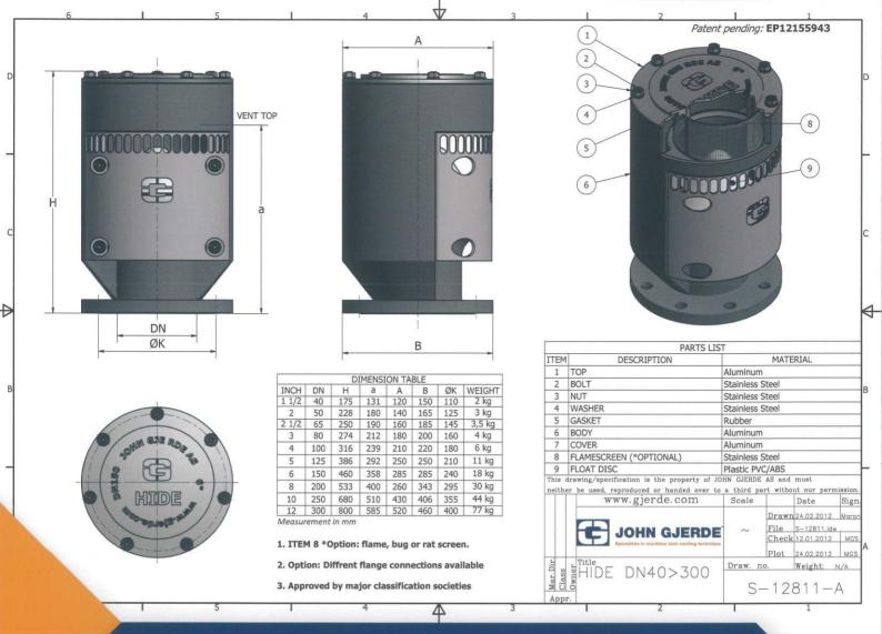
The new patented **HIDE** aluminum tank vent check valves of John Gjerde combines light weight, compact design and high flow capacity.
