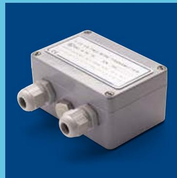
The MAS2600 is a 2-wire 4-20 mA level transmitter consisting of a transducer and an amplifier connected via a 6-core vented cable. The amplifier is housed in a sea water-resistant polyester casing (IP56).
